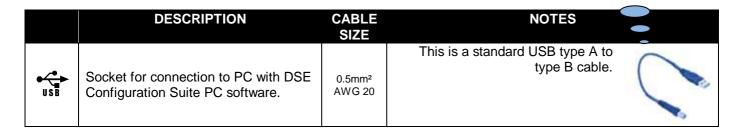
**A**NOTE:- The USB connection cable between the PC and the DSE331 module must not be extended beyond 5m (5yds). For distances over 5m, it is possible to use a third party USB extender. Typically, they extend USB up to 50m (yds). The supply and support of this type of equipment is outside the scope of Deep Sea Electronics PLC.
