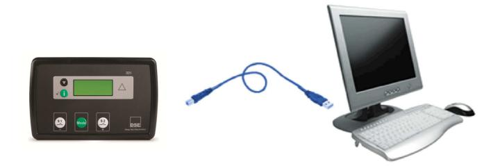
**A**NOTE:-<u>The DC supply must be connected to the module for configuration by PC.</u>
